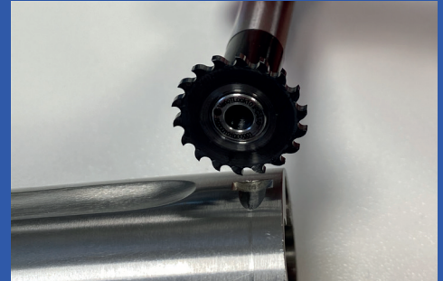
Our SlitEX machines many different types of slots into pistol slides
