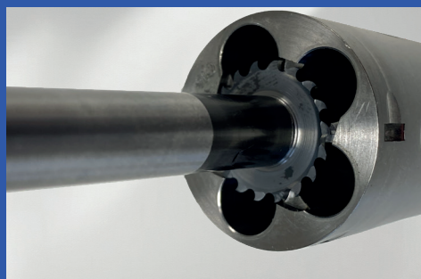
SlitEX can be used to machine the inside of a cylinder
