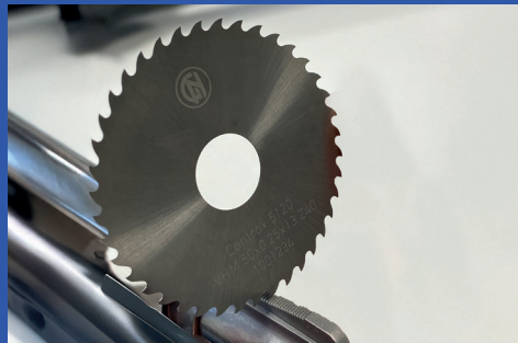
Slitting saw can be used to machine slots in the front sight
