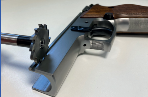
SlitEX can be used for the slot on the side of pistol frames
