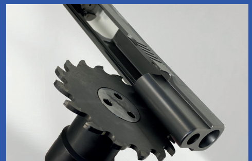
A larger SlitEX to slot the underside of a pistol slide
